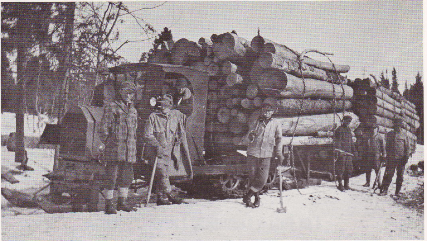
The Linn tractor, introduced shortly after World War I, signaled growing mechanization in the foothills lumber industry.
